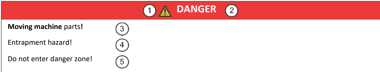
Figure 1: Structure of a warning notice
